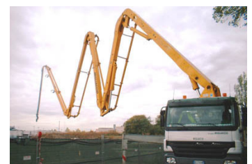
Concrete pump extensible arm
