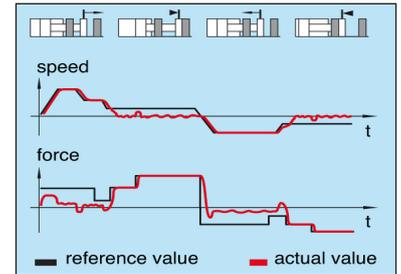
Fig. 2 - Motion profile example
