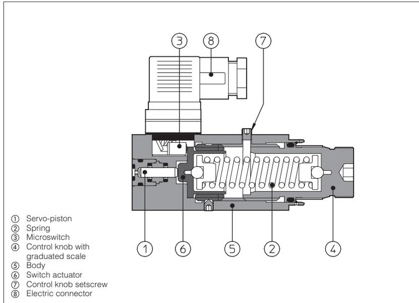
**SMAP** are hydro-electric pressure switches with fixed switching pressure differential. The mechanical microswitch with gold plated contacts grants high reliability and long life service.
