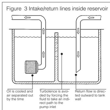
In the reservoirs having a big capacity, commonly internal baffles are provided for the separation of the oil return area from the pumps intake, in order to brake the swirling movement of the liquid and to allow the setting of solid suspended particles and also of the water, if any.
