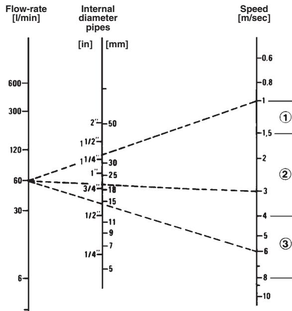
Example: with flow rate of 60 l/min and flow speed of 1,3 and 6 m/sec the recommended internal diameter of the pipe is 33,20 and 14 mm respectively.
