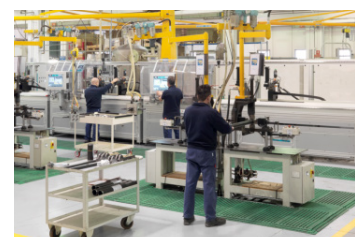
Cylinder's automatic test benches
