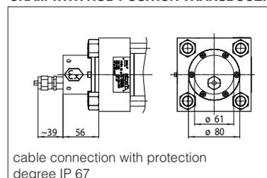
cable connection with protection degree IP 67
