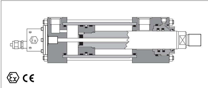
CKA cylinders are derived from standard CK (tab.B137) with certification according to ATEX 2014/34/EU. They are designed to limit the external surface temperature, according to the certified class, to avoid the self-ignition of the explosive mixtures potentially present in the environment. CKAM servocylinders are equipped with ex-proof built-in digital magnetostrictive position transducer, ATEX certified.
