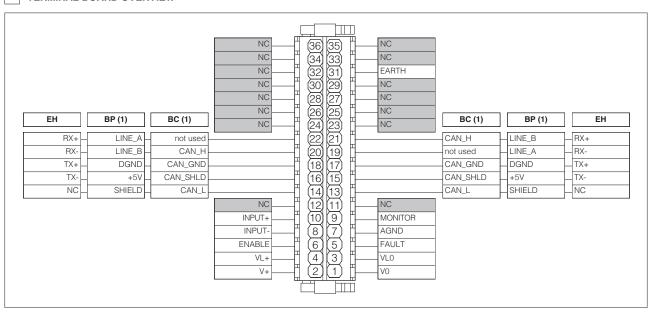
(1) For BC and BP executions the fieldbus connections have an internal pass-through connection
