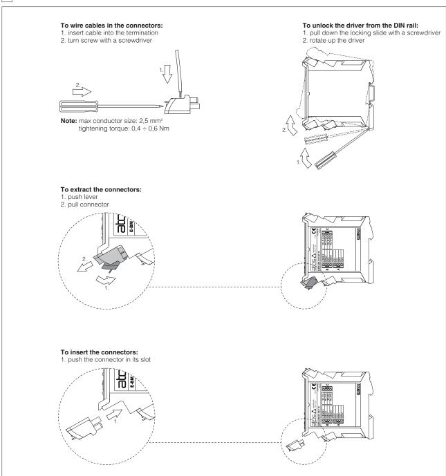
Note: all connectors are supplied with a mechanical coding. This feature ensures a unique insertion of each connector in the own slot (eg. connector A can not be inserted into connector slot of B, C, F, G, H)
