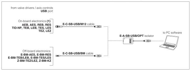
(1) USB port is not available for on-board TID-BC valve drivers
