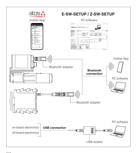
Atos CONNECT is a free iOS / Android mobile App available in the respective App stores, while E-SW-SETUP and Z-SW-SETUP programming software are developed for Windows and free downloadable at www.atos.com in MyAtos download area.
