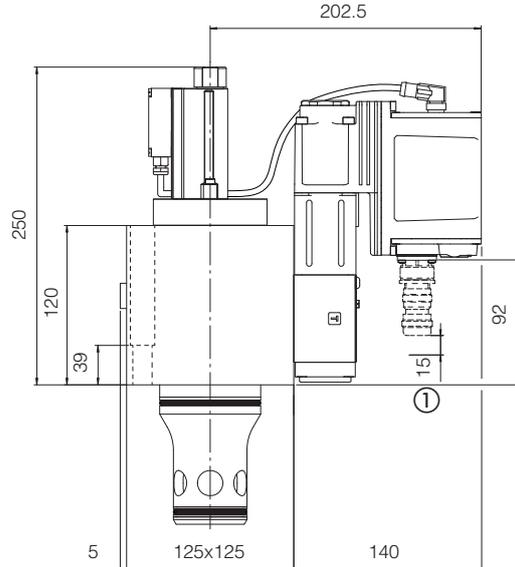
① Space to remove the 7 or 12 pin main connector. For main and communication connectors see section 9, 10
