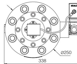
① Space to remove the 7 or 12 pin main connector. For main and communication connectors see section 9, 10
