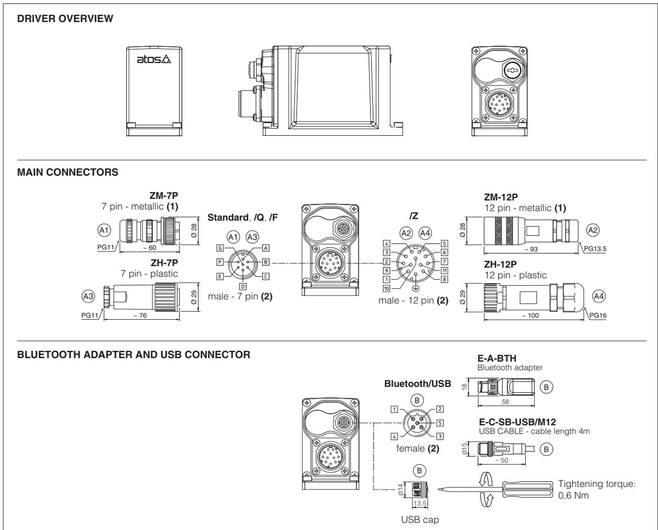
(1) Use of metallic connectors is strongly recommended in order to fulfill EMC requirements (2) Pin layout always referred to driver's view
