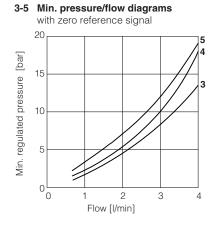
**Note**: the presence of counter pressure at port T can affect the pressure regulation and the minimum pressure
