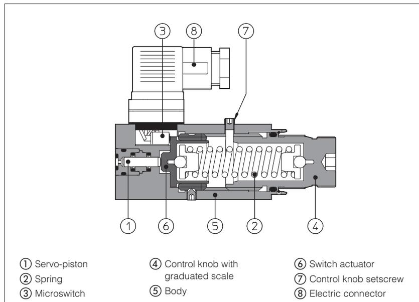
**SMAP** are hydro-electric pressure switches with fixed switching pressure differential. The mechanical microswitch with gold plated contacts grants high reliability and long life service.
