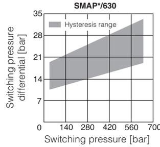
The diagrams show, the switching pressure difference (hysteresis) between the switching positions of the pressure switch electric contacts.
