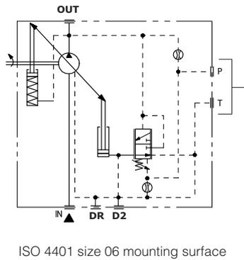
**GM General purpose compensator with ISO 4401 size 06 mounting surface**
