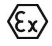
II 1G Ex ia IIC T6 Ga or II 1G Ex ia IIC T5 Ga or I M1 Ex ia I Ma (only /M version)
