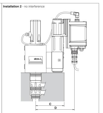
**C** = Max manifold dimension to avoid interference with the main connector, see below table
