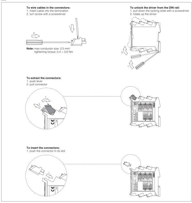
Note: all connectors are supplied with a mechanical coding. This feature ensures a unique insertion of each connector in the own slot. (e.g. connector A can not be inserted into connector slot of B,D,E,F)
