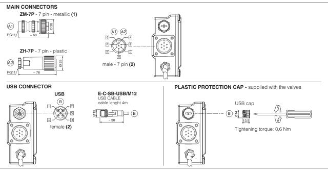
(1) use of metallic connectors is strongly recommended in order to fulfill EMC requirements
