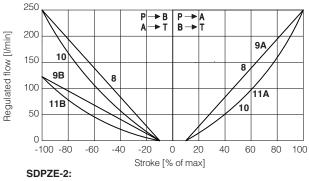
**SDPZE-2: 8** = L5 **9A** = DL5 ( $P \rightarrow A$ ,  $A \rightarrow T$ ) **11A** = D5 ( $P \rightarrow A$ ,  $A \rightarrow T$ ) **10** = S5 **9B** = DL5 ( $P \rightarrow B$ ,  $B \rightarrow T$ ) **11B** = D5 ( $P \rightarrow B$ ,  $B \rightarrow T$ )
