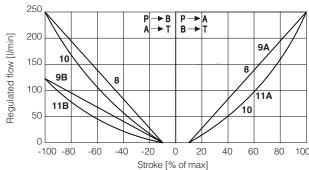
**SDPZE-2: 8** = L5 **9A** = DL5 (P $\rightarrow$  A, A $\rightarrow$  T) **11A** = D5 (P $\rightarrow$  A, A $\rightarrow$  T) **10** = S5 **9B** = DL5 (P $\rightarrow$  B, B $\rightarrow$  T) **11B** = D5 (P $\rightarrow$  B, B $\rightarrow$  T)
