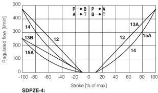
**12**=L5 **13A**=DL5 (P $\rightarrow$ A, A $\rightarrow$ T) **15A**=D5 (P $\rightarrow$ A, A $\rightarrow$ T) **14**=S5 **13B**=DL5 (P $\rightarrow$ B, B $\rightarrow$ T) **15B**=D5 (P $\rightarrow$ B, B $\rightarrow$ T)
