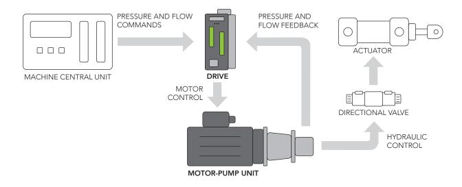
An angular position transducer, integrated in the motor-pump unit, provides the drive with the information on the flow rate generated by the pump. A pressure transducer installed on the pump outlet provides the information on the actual pressure of the hydraulic user line.
