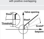
Double solenoid directional control valve, 3 positions with positive overlapping
