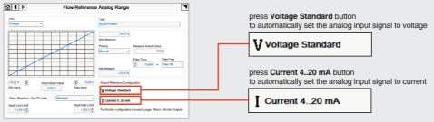
REMARK: Voltage Standard or Current 4..20 mA buttons do not act on Monitor output signal configuration! For Monitor output signal configuration browse to page Others - Monitor Output
