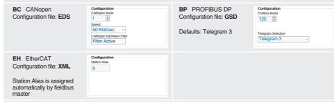
• press Memory Store button and in Fieldbus Parameters press Store User button to save new setting into the driver (see 3.4)
