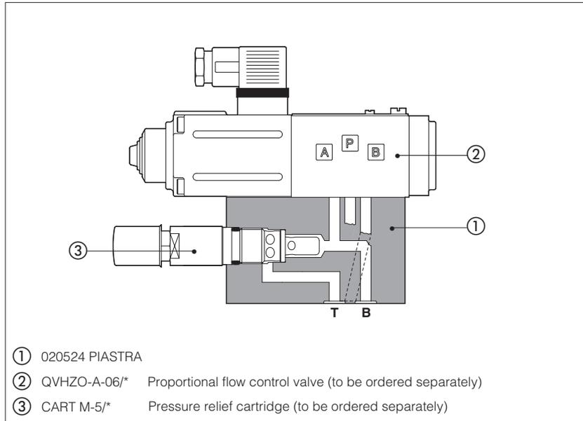
SP-020524 PIASTRA is a ISO 4401 size 06 special modular plate providing a pressure compensated meter-in flow regulation in standard multistation subplated type BA\*
