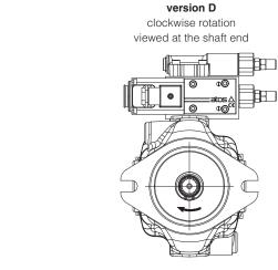
Pumps with clockwise rotation (**D**) have the IN and OUT as shown in all representation of catalogue
