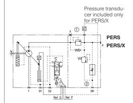
P/Q control integrates the alternate pressure and flow regulation with the electronic max power limitation.
