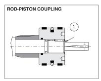
The rod and piston are mechanically coupled by a threaded connection in which the thread on the rod is at least equal to the external thread KK, indicated in the table 7. The piston is screwed to the rod by a pre-fixed tightening torque in order to improve the fatigue resistance. The stop pin ① avoids the piston unscrewing.
