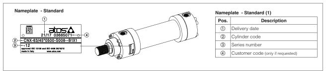
Notes: (1) The position of the nameplate on the rear or front heads can change due to the cylinder overall dimensions
