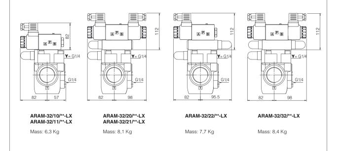
Overall dimensions refer to valves  ${f DC}$  voltage, with connectors type 666
