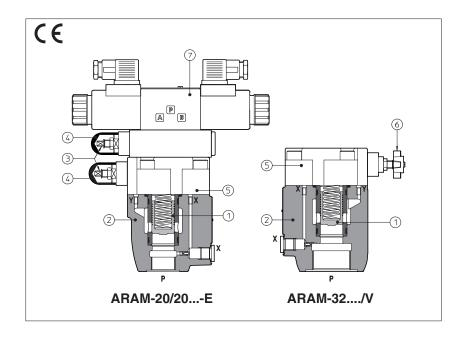
**ARAM** are two stage pressure relief valves with balanced poppet, designed with threaded ports for in-line mounting.
