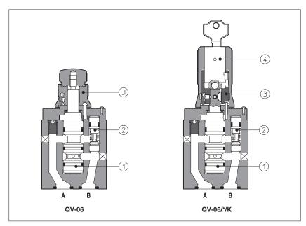
**QV** are flow control valves with pressure compensator ①: the controlled flow rate is independent of pressure variations.
