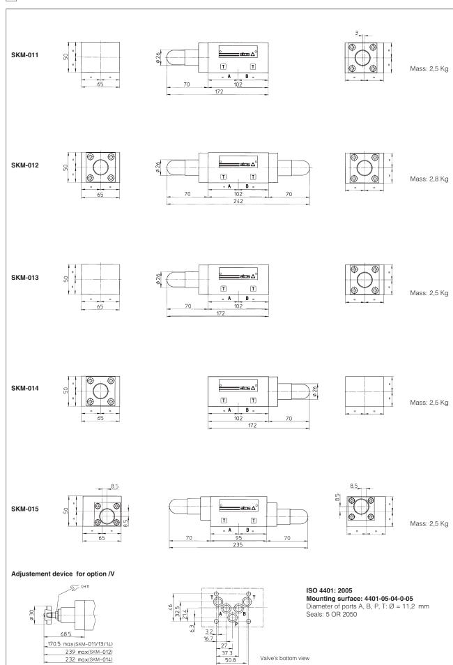
Fastening bolts: nº 4 socket head screws M6. The length depends on number and type of modular elements associated.
