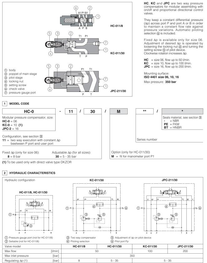
(1) The Δp for single flow path is fixed at 8 bar or is adjustable between 5 and 35 bar; it corresponds to values of total Δp across the valve of 16 bar or between 10 and 70 bar. Threaded plugged ports Pp and P1 are suitable for pressure adjustment or check of Δp value for single flow path (reading difference between Pp and P1 values).
