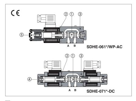
Spool type, two or three position direct operated valves with high performance threaded solenoids.
