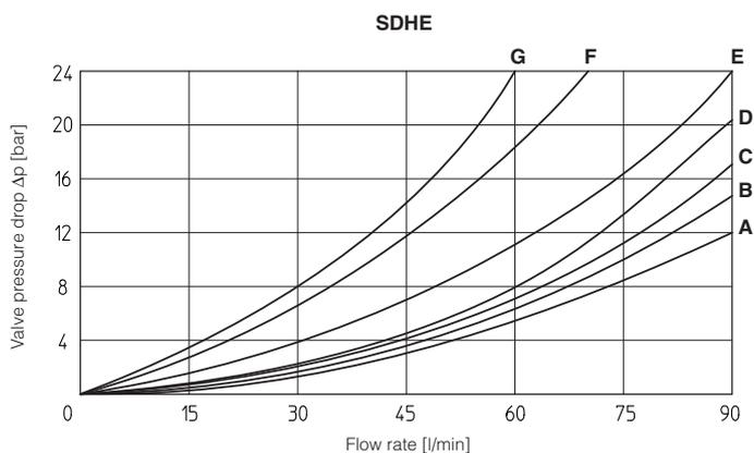
**8 OPERATING LIMITS** based on mineral oil ISO VG 46 at 50°C
