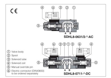
Spool type, two or three position direct operated solenoid valves size 06 in low leakage and compact execution with reduced solenoids dimensions, ideal for hydraulic systems assisted by accumulators.
