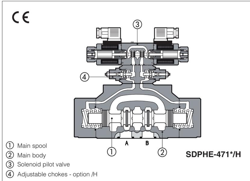
Spool type, pilot operated directional solenoid valves available in three or four way configurations.
