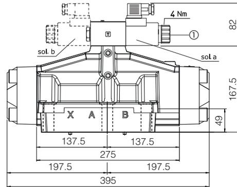
Overall dimensions refer to valves with connectors type 666
