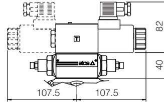
**Stroke adjustment device for option/S**
