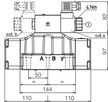
Overall dimensions refer to valves with connectors type 666
