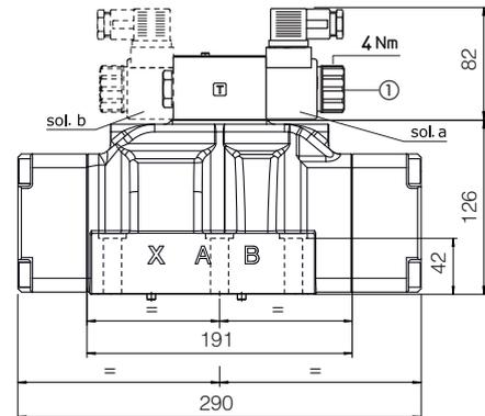
Overall dimensions refer to valves with connectors type 666
