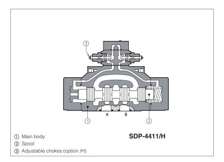
Spool type hydraulic operated directional valves in three or four way, two or three position.
