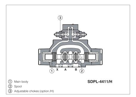
Spool type hydraulic operated directional valves available in three or four way configurations.
