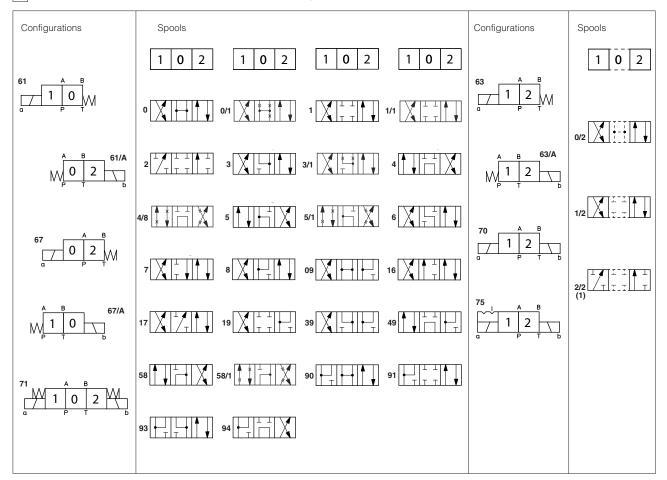
For spool type 2 and 2/2 port T of the valve must be connected to tank if the operating pressure exceed the max T pressure reported at section 4 (1): not available for configuration 75
