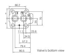
ISO 6264: 2007 Mounting surface: 6264-08-13-1-97 Fastening bolts: 4 socket head screws M16x50 class 12.9
