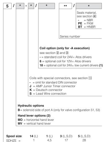
(1) Select coil voltage /18 in case of electronic drivers not supplied by Atos, with power supply 24 VDC
