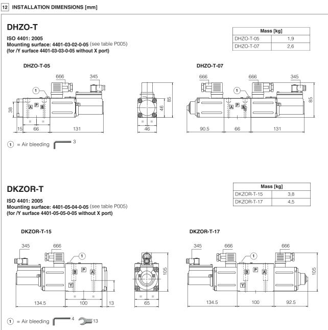
Note: for option /B the solenoid and the LVDT transducer are at side of port A
