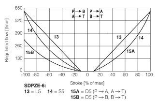
Note: Hydraulic configuration vs. reference signal for configuration 71 and 73 (standard and option /B)
