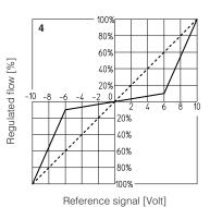
Hydraulic configuration vs. reference signal:
