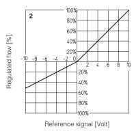
T3, T5 and T7 spool types are specific for fine low flow control in the range from 0 to 60% (T5) and 0 to 40% (T3, T7) of max spool stroke.
