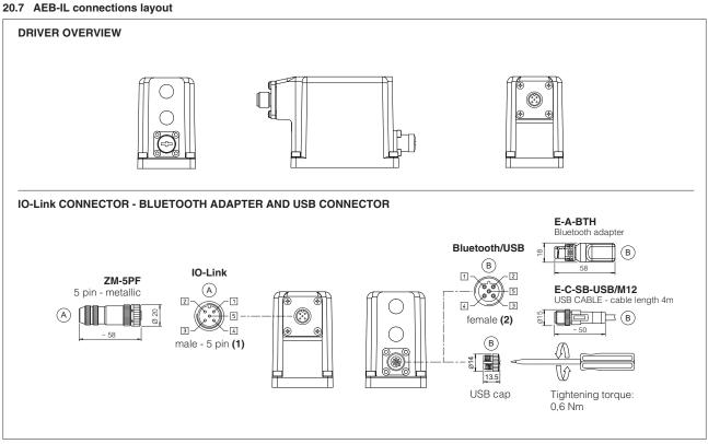
(1) Use of metallic connectors is strongly recommended in order to fulfill EMC requirements
