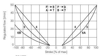
**SDHZE**  $\begin{aligned} \textbf{6A} &= D5 \ (P \rightarrow A, \ A \rightarrow T) \\ \textbf{6B} &= D5 \ (P \rightarrow B, \ B \rightarrow T) \end{aligned}$ **4** = L5 **5** = S5
