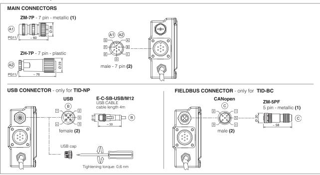
(1) use of metallic connectors is strongly recommended in order to fulfill EMC requirements (2) pin layout always referred to driver's view
