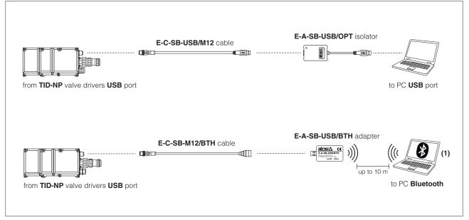
(1) If PC has not built-in Bluetooth, use standard USB to Bluetooth dongle compatible with E-A-SB-USB/BTH specification (please refer to STARTUP-BLUETOOTH guide)
