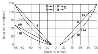
SDPZE-2: **9A** = DL5 (P $\rightarrow$ A, A $\rightarrow$ T) **11A** = D5 (P $\rightarrow$ A, A $\rightarrow$ T) **8** = L5 **10** = S5 **9B** = DL5 (P  $\rightarrow$  B, B  $\rightarrow$  T) **11B** = D5 (P  $\rightarrow$  B, B  $\rightarrow$  T)
