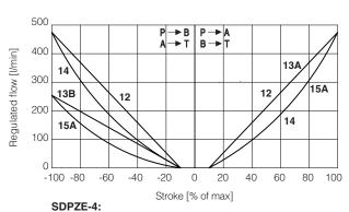
**12**=L5 **13A**=DL5 (P $\rightarrow$ A, A $\rightarrow$ T) **15A**=D5 (P $\rightarrow$ A, A $\rightarrow$ T) **14**=S5 **13B**=DL5 (P $\rightarrow$ B, B $\rightarrow$ T) **15B**=D5 (P $\rightarrow$ B, B $\rightarrow$ T)
