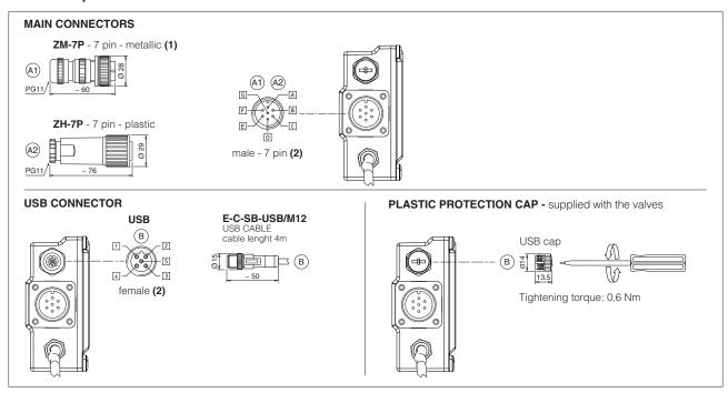
(1) use of metallic connectors is strongly recommended in order to fulfill EMC requirements
