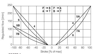
SDPZE-2: **5A** = DL5 (P $\rightarrow$ A, A $\rightarrow$ T) **7A** = D5 (P $\rightarrow$ A, A $\rightarrow$ T) **4** = L5 **5B** = DL5 (P  $\rightarrow$  B, B  $\rightarrow$  T) **7B** = D5 (P  $\rightarrow$  B, B  $\rightarrow$  T)
