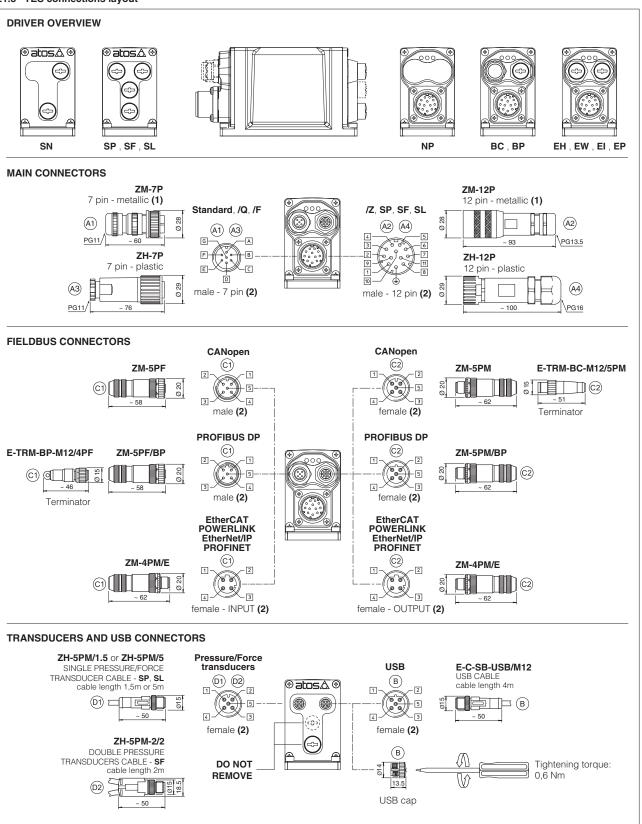
(1) Use of metallic connectors is strongly recommended in order to fulfill EMC requirements (2) Pin layout a
